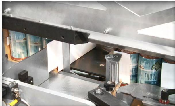
The **Vantra IM** cartoner/tray packer provides a highly versatile single platform solution designed with a hygienic sheet metal frame and standoff bearing mounts.
