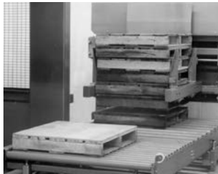
Multi-size pallet dispenser with roller conveyor
