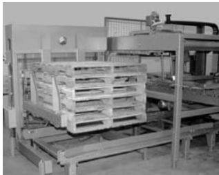
Pallet dispenser with 2 chain conveyor
