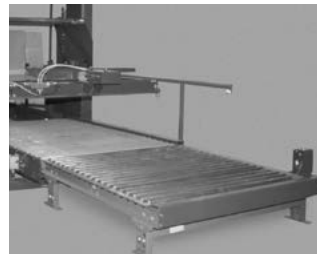
5' gravity discharge roller conveyor
