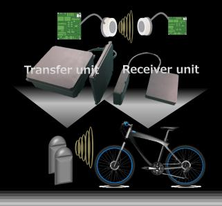
Even if shifting coil position, electricity can be transferred with high efficiency. OMRON 2nd-Resonance technology adjust to optimal frequency when the coil position shifts greatly.
