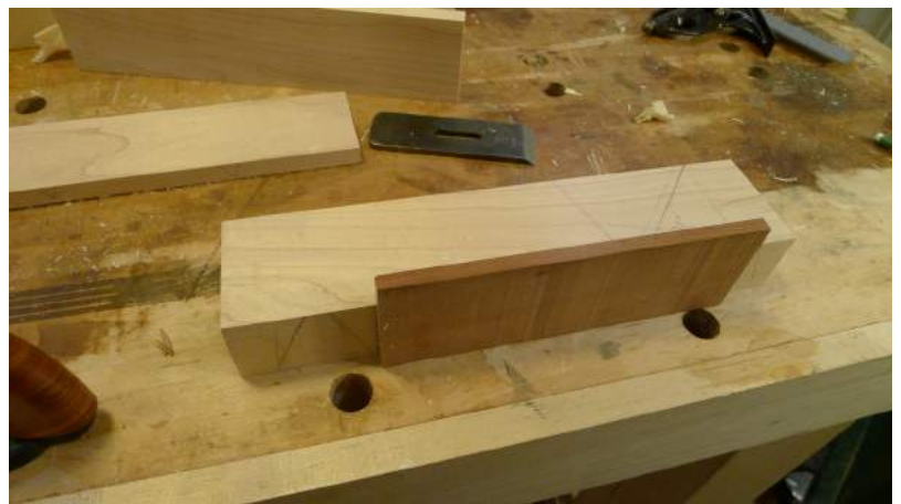
Fitting the insert into a shallow mortise in the center piece.
