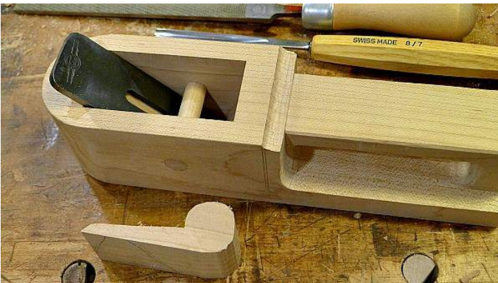
The wedge was made from the piece cut out for the throat of the plane.
