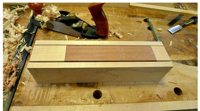
The sole insert glued into the center piece, trimmed and planed and ready for subsequent steps.
