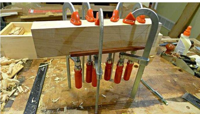
The center piece is glued and clamped together. Once set, it will be trimmed and planed.
