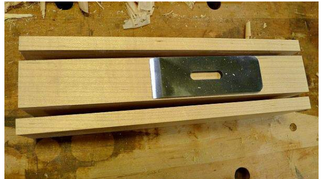
Front of the plane-to-be is on the left. The blank plane body, with the sides sawn and the central piece a fat 1/16" thicker than the iron is wide.
