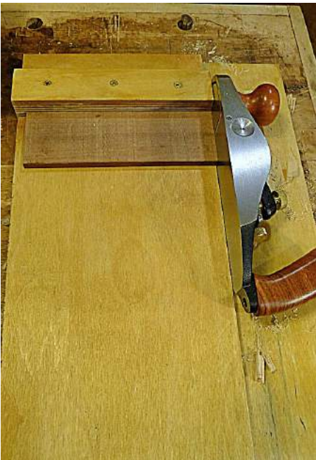
Squaring off the sole insert with a shooting board.
