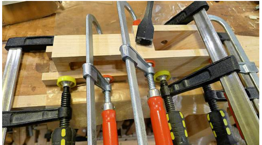
I clamped the ramp section to my workbench, then glued one side and then the other to the body of the plane.
