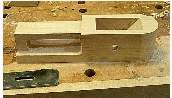
I accomplished this initial shaping on the bandsaw.
