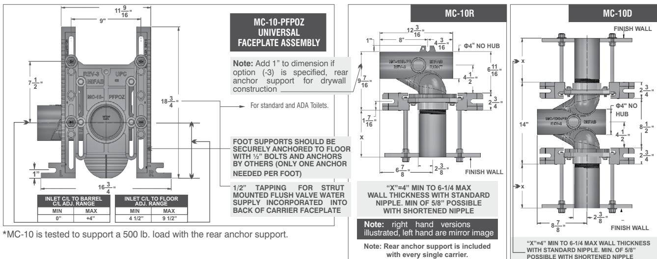
\*MC-10 is tested to support a 500 lb. load with the rear anchor support.
