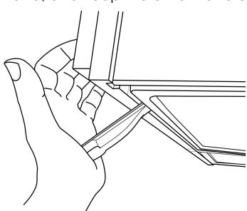
Push the Removal tool in between the light and the cabinet (as shown) until the light pops off.
