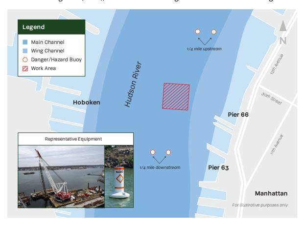
The Hudson River Ground Stabilization (HRGS) project will fortify a section of the riverbed to enable tunnel boring machine operations for the future Hudson River Tunnel. To ensure the safety of boaters and construction crews on the water, The United States Coast Guard (USCG) has issued the following **Notice to Mariners** (available at <u>USCG.mil</u>):
