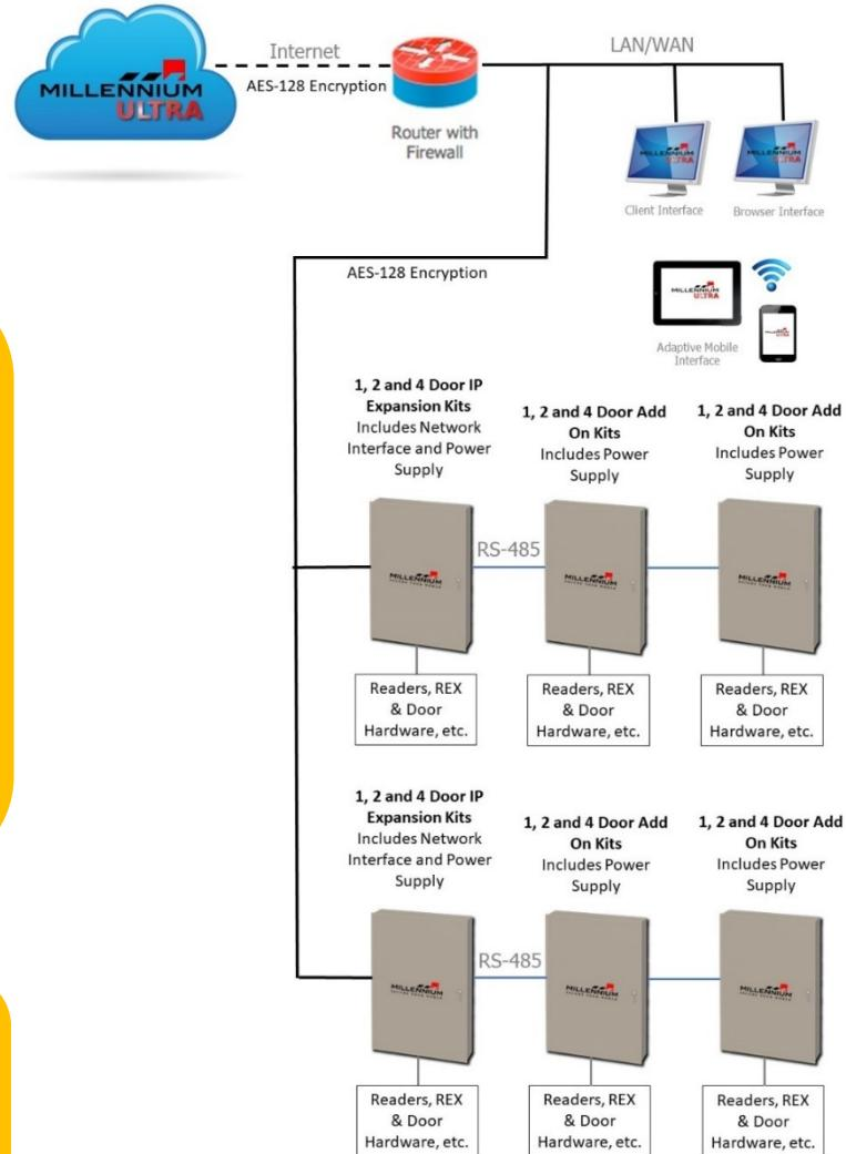
Diagram shows layout using pre-engineered systems. Cloud-hosted is also available with our engineered products.
