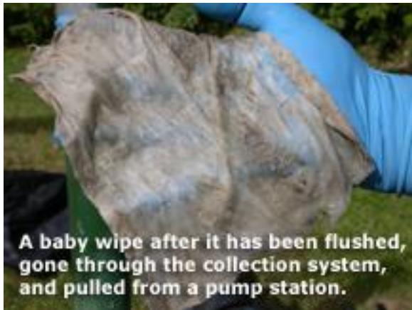
**A baby wipe after it has been flushed, gone through the collection system, and pulled from a pump station.**
