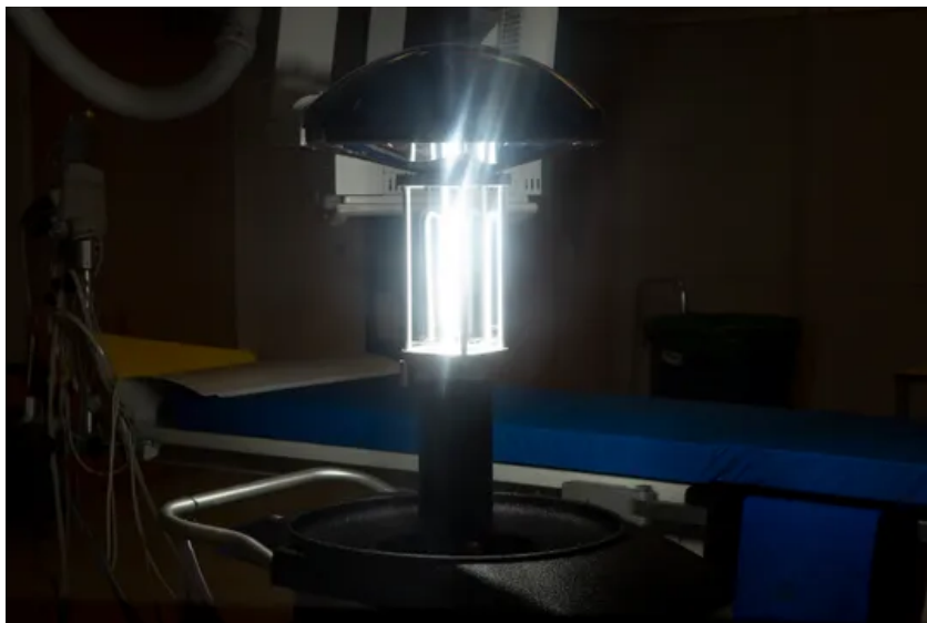
A Xenex LightStrike Germ-Zapping robot uses pulsed xenon ultraviolet light to disinfect a room at NCH Downtown Baker Hospital in Naples on Tuesday, February 4, 2020. NCH now has three of the robots, which help to decrease infection rates by disinfecting rooms after the rooms are manually cleaned. (Photo: Alex Driehaus/Naples Daily News/USA TODAY - FLORIDA NETWORK)
