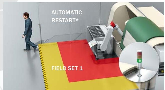
**3** The robot stops when the worker enters the protective field.
