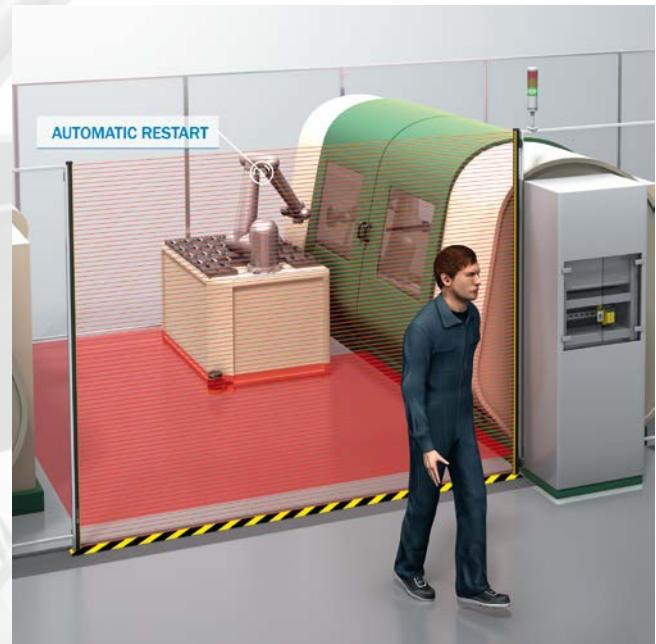
3 The secondary protective device detects whether people are located in the protective field and ensures that the robot remains safely stopped as long as the worker is in the hazardous area.
