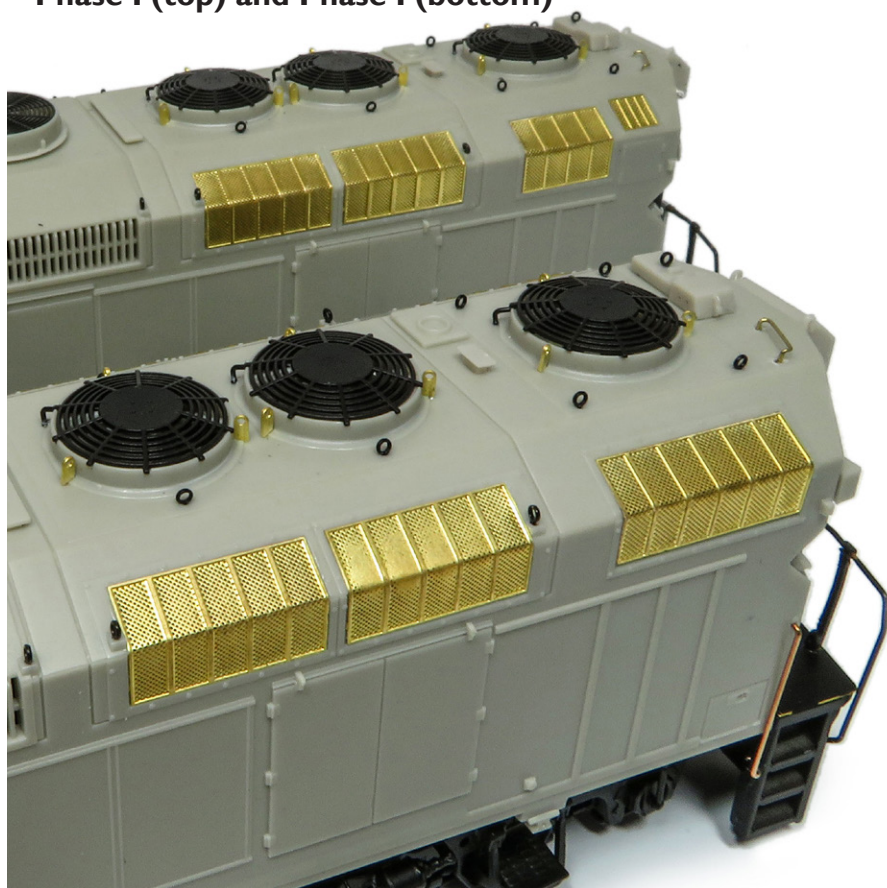
Eroded Metal Grills and Rooftop details Phase I (top) and Phase I (bottom)
