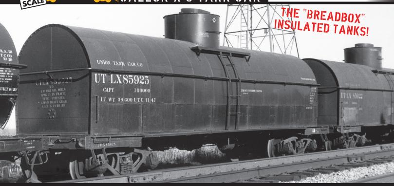
UNION TANK CAR MODIFIED A GROUP OF X-3s THROUGH THE ADDITION OF HEATER COILS OUTSIDE OF THE TANKS WITH WAGON-STYLE INSULATION AND JACKETING. THESE HIGHLY DISTINCTIVE AND INTERESTING CARS WERE PRIMARILY FOR THE TRANSPORT OF TRANSFORMER OIL, USED TO INSULATE AND COOL TRANSFORMERS. THESE CARS, NEVER BEFORE OFFERED IN STYRENE, COULD BE SEEN ANYWHERE IN THE US FROM THE 1920s INTO THE 1960s.
