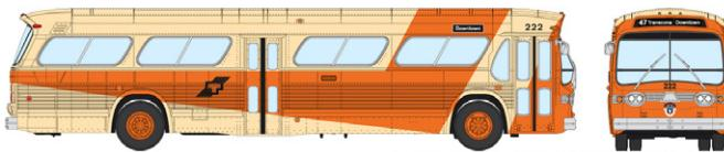
Features: Left-side Emergency Door, Partial EIP package, 4-window exit door, Late-style engine door
