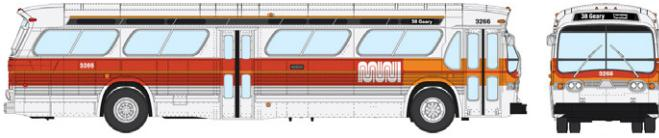
Features: Rear EIP package, 4-window exit door, Late-style engine door, Rubber front bumper
