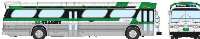
*Features: A/C, Rear EIP, 4-window Rear Exit Door, Sealed Windows, Late-style Engine Door, Standee Windows*
