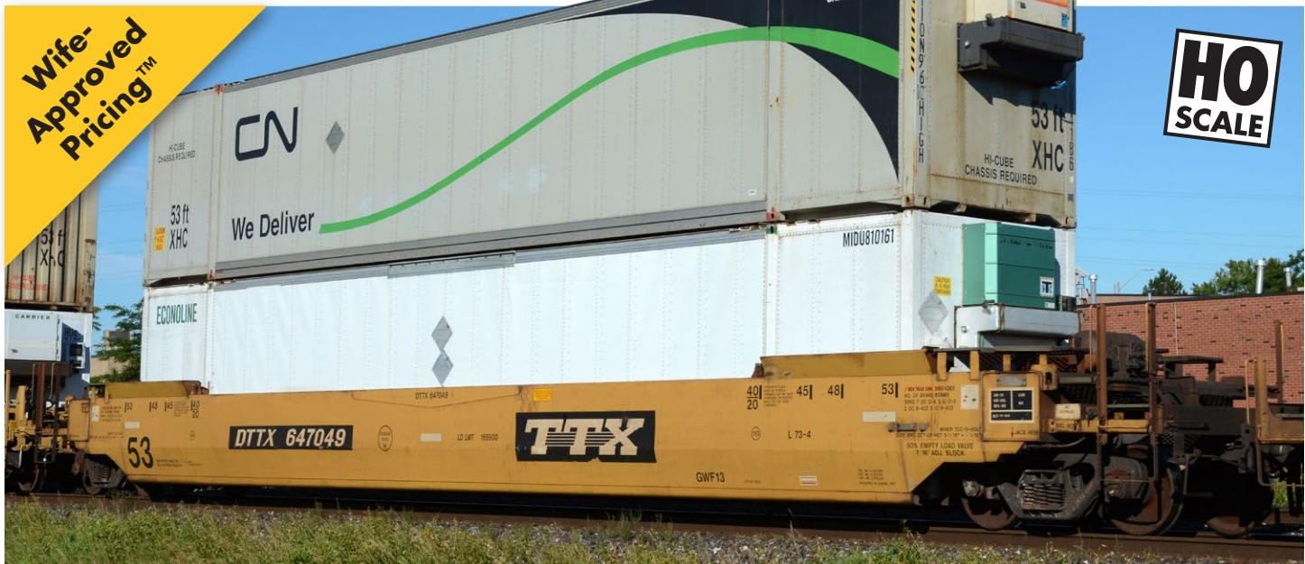
The Gunderson 53' single-unit double-stack well car is the latest iteration of the famous Husky-Stack and every intermodal train includes at least three or four cars of this type. This is accompanied by a newly tooled 53' high-cube container with riveted sheet/post sides and optional heater box/fuel tank.
