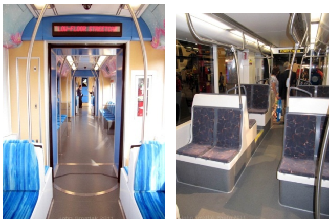
FIGURE 1-9 100 Percent Low-Floor Interior
