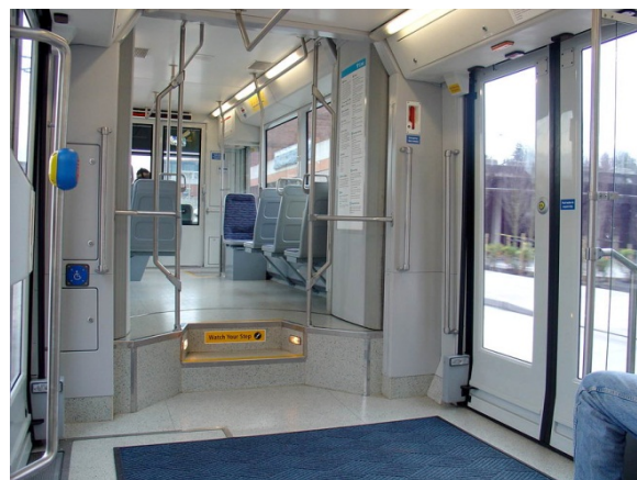
FIGURE 1-10 Partial Low-Floor Interior
