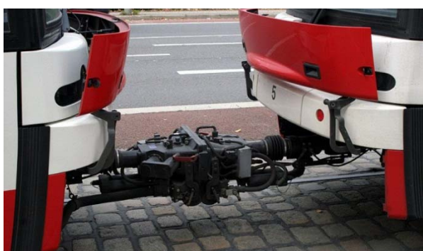
Full couplers (retractable type, with movable carbody skirt) in Dortmund, Germany.
