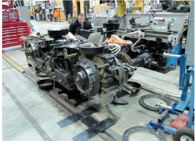
On trucks with inboard frames and drive train components, removal of wheel tires is relatively straightforward, although some designs may have braking components outboard of the wheels that will also need to be removed.
