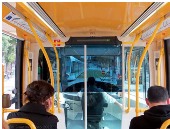
FIGURE 1-11 Clear Cab Partition Wall
