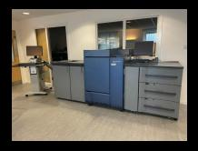
Bizhub Press C1085, PF-707 A3 Deck, RU-511 Relay Unit, FS-532 Finisher, IC-308 External EFI Fiery, C-832k B-850K
