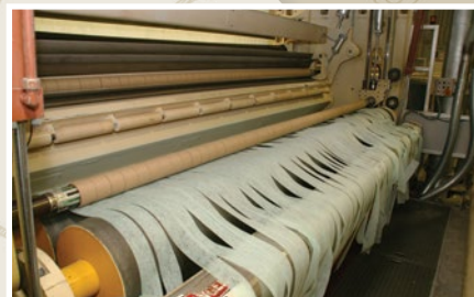
Locked-core shaft in two-drum winder
