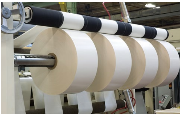
Goldenrod 1250 DFX shaft on duplex winder
