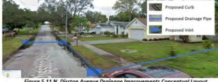
Figure 5.11 N. Disston Avenue Drainage Improvements Conceptual Layout
