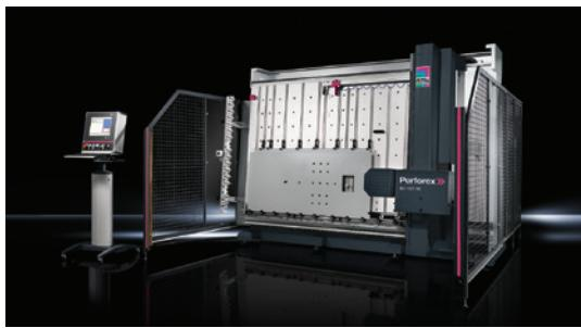
Our state-of-the-art Perforex machine can modify stainless steel or carbon steel wallmount, junction boxes, and TS enclosures per your specifications. We'll apply standard holes, and cutouts for both enclosures and mounting panels.
