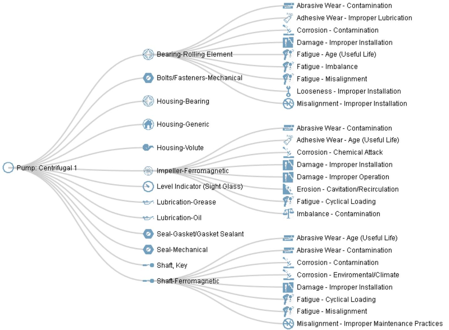
Figure 1: Centrifugal Pump, Parts and sample failure modes.
