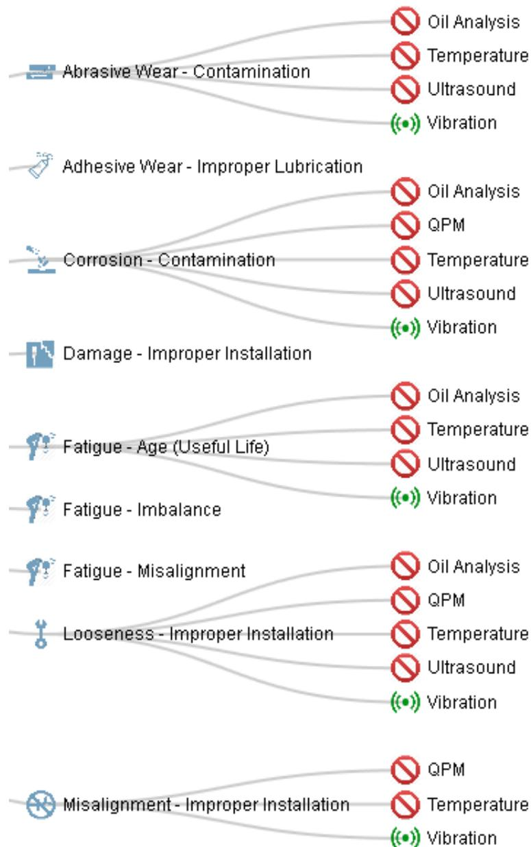
Figure 2: Sensory Measures useful in detecting defects leading to particular failure modes.
