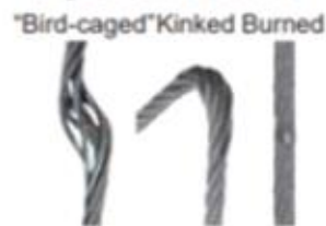
Fig. B: Cable Defects
