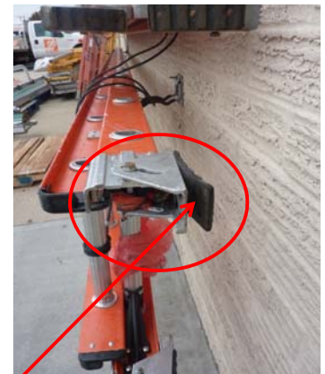
Damaged Safety Shoe : Rubber Pad Damaged
