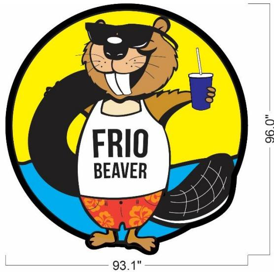
Specs: One welded channel logo w/ polycarbonate face and LED's - self contained.
