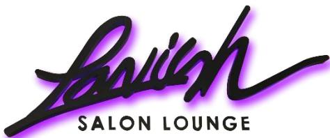
**Illuminated Reverse** – LED Illuminated Reverse Channel Letters feature an aluminum face and return, but a clear polycarbonate back allowing the light to create a halo effect around the letters or logos.
