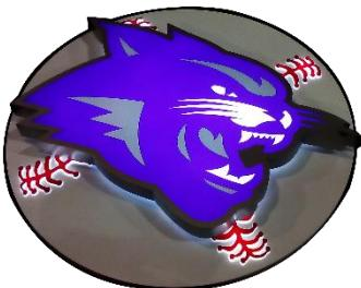
**FRONT/BACK LIT** – This form of sign can fall under any of the above categories, but also has light shining through the back, similar to a reverse channel sign. The face is acrylic, and the backs are typically clear polycarbonate. Two different colors of LEDs can be accomplished by adding a false back – a divider – in the can.
