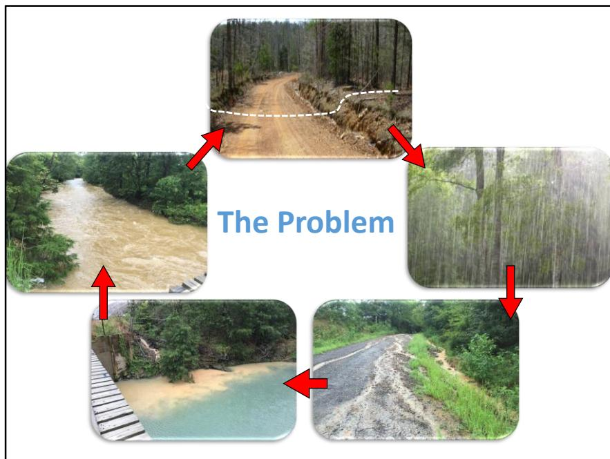
Eroding unpaved roads are one of the greatest sources of sediment to our streams, rivers and lakes.
