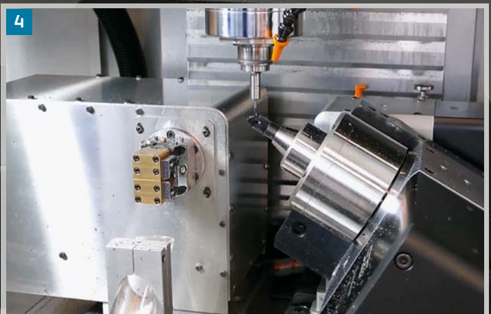
Machining with 5 axes (4 simultaneous axes)
