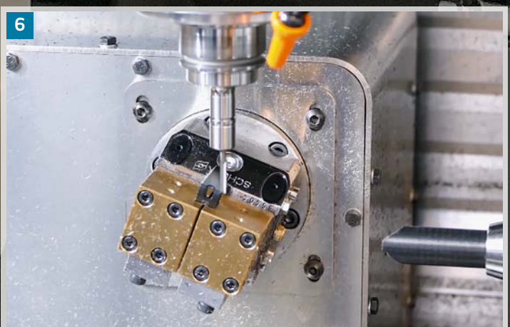
6 th face machining with the pickup unit
