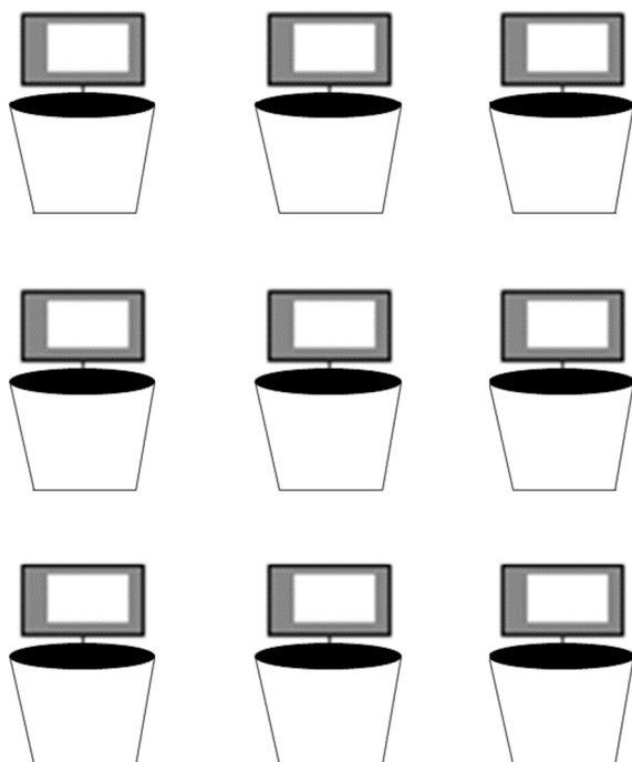
Fig. 1. Grid pattern design of the Kromekote® card collectors affixed to horizontal metal plates in vermiculite filled pots. Each nozzle by pressure combination was applied over 9 cards in a 3 by 3 pattern.
