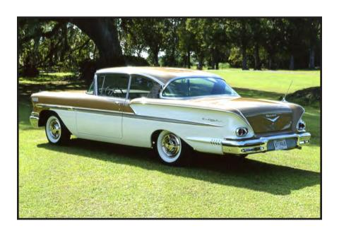
Chevrolet made big changes to its cars in 1958, including a new X-frame, 117.5" wheelbase, exterior sheet metal and interiors. A standard V-8 engine selection on '58 Chevys brought with it 185-horsepower, but more powerful engines could be had offering up to 290-horsepower.
