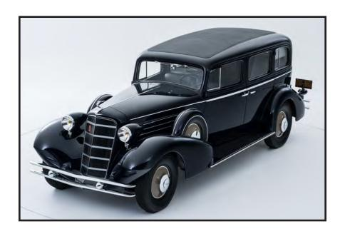
1934 would be an eventful year for Cadillac, introducing sleek new sheet metal and noteworthy mechanical improvements. '34 Cadillacs were the first in the industry to move the spare tire out of site and into the trunk, and the new "knee-action" independent coil spring suspension provided outstanding riding comfort.
