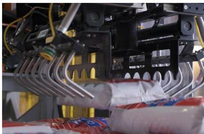
3. During drop-down initially only the gripper fingers open.
