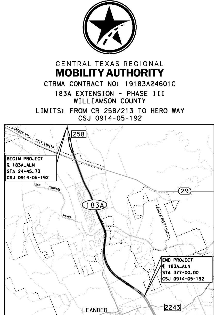
FOR THE CONSTRUCTION OF A TOLLWAY FACILITY CONSISTING OF CONCRETE PAVEMENT, ASPHALT PAVEMENT, BRIDGES, RETAINING WALLS, GRADING, CULVERT STRUCTURES, STORM SEWERS, PEDESTRIAN FACILITIES, WATER QUALITY, DETENTION FACILITIES, SIGNING, STRIPING, SIGNALS AND ILLUMINATION.
