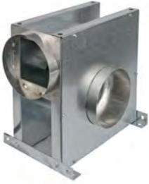
A 90° inline or roof mounted exhaust fan for laundry applications. The housing is constructed of G90 galvanized steel and the dynamically balanced backward inclined or backward curved impeller is constructed in 5052 aluminum.
