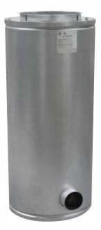
The PSS has a 3" high temperature fiber-insulated double-wall, which provides a UL/ULC classified 2-hour fire-rated shaft eliminating the need for field fabricated duct work and a separate fire-rated shaft construction thus reducing material, labor, and installation costs. The PSS is made in the USA and includes a limited lifetime warranty with engineering technical support.
