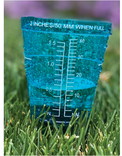
Example of a water gauge from a Water Audit Kit. Place 3-5 gauges in a station to test sprinkler output and coverage.
