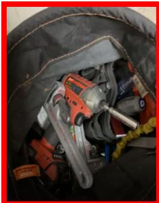
There should not be any energized tools in job bags. When placing battery operated tools in your bag, make sure the battery is removed to prevent inadvertent start up.
