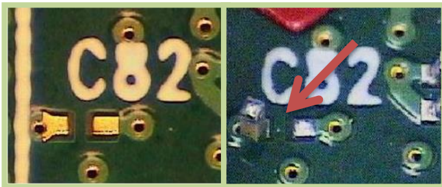
Soldermask clearance connecting a via to a component land, resulting in a tombstone defect.
