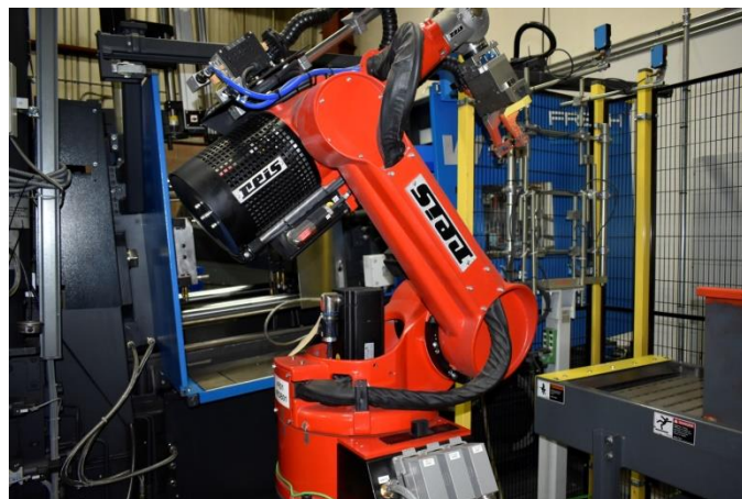
Robotic Arm: Automatically removes part and lays it on cooling conveyor.
