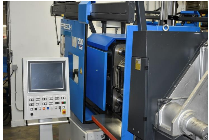
Automated Setting Control Panel: Temperature, Pressure, Spray and other settings are as easy as push buttons.
