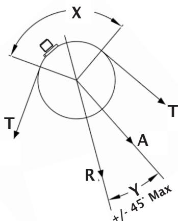
To size and select the correct load rating of the ISR, the total load on the sensing roll must be calculated. This load consists of the tension components in the sensing plane. Using the known maximum tension and angles as shown, apply the equation below to calculate the actual load.
