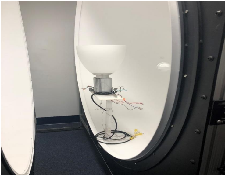
Photo 2 (above) – Integrating Sphere with Pathway Model P31 Fixture Set Up for Testing
