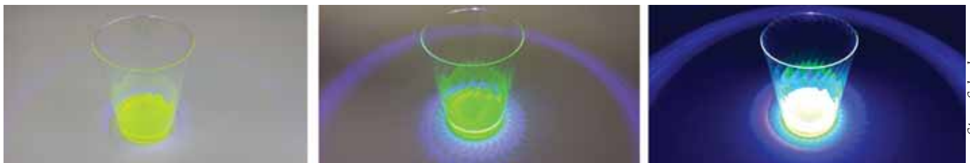
Figure 7: Conventional green antifreeze with dye may be easy to see under UV in natural light, but it gets even better when the lights are turned down. Otherwise much of the natural / ambient light will wash out some of the fluorescence, making it more difficult to see.
