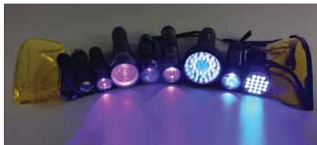
Figure 9: Not all "UV flashlights" put out the same wavelengths of light, and therefore may or may not be best suited to fluoresce the dye you're working with. That's why we recommend having several different UV flashlights of varying wavelengths. These range from 365 nm (on left, almost invisible), up to 450 nm (a very "blue" color).
