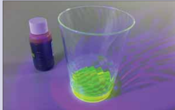
Figure 14: A comparison of coolant dye, both concentrated and mixed with conventional antifreeze. It looks dark brown in the bottle, but when properly mixed it's really bright yellow/green!
