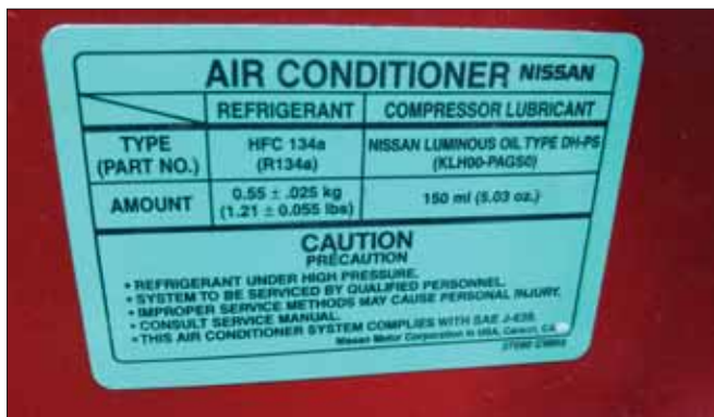
Figure 8: This Altima label says it uses "Nissan Luminous Oil Type DH-PS", but there's another hidden clue. If you shine a UV light onto the label, it glows!
