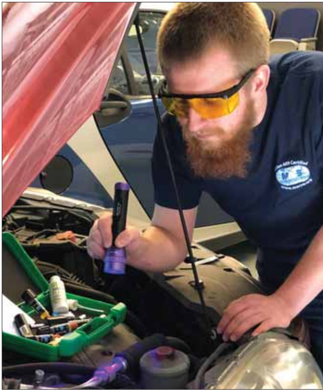
Figure 3: Popular dye kits come with everything you need: pre-measured dosage bottles, a way to add the dye, a UV light and glasses that make it easier to find leaks.
