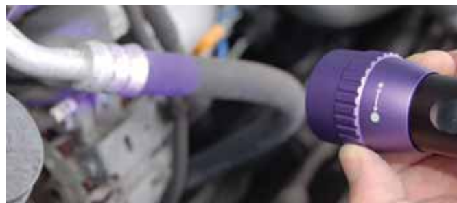
Figure 10: It's easy to focus the light beam on many modern flashlights by simply rotating or sliding the lens. Some UV flashlights can also do this, which spreads the light out evenly.
