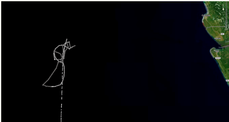
Figure 9: AIS spoofing by Blazers (IMO: 9307645)
