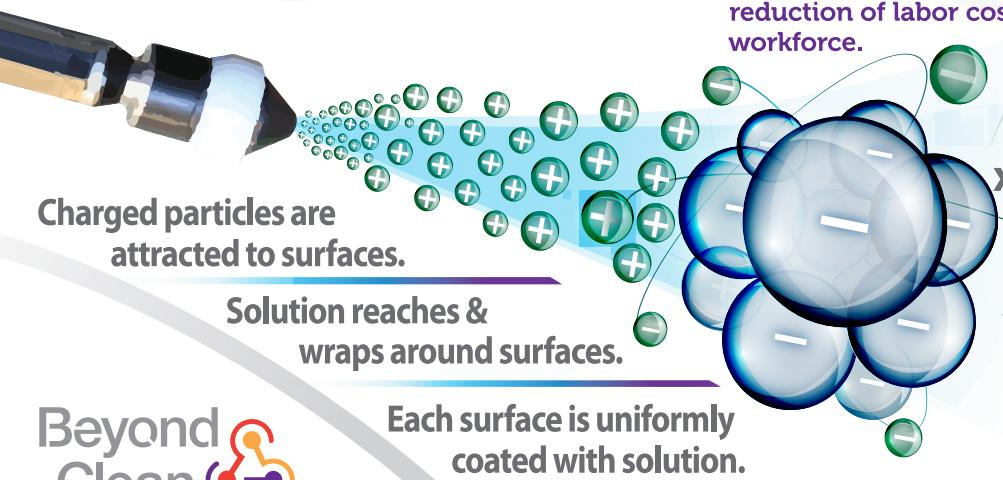
After the spray is applied, the sanitizing agent works to disinfect the objects and surfaces. For this reason, electrostatic spray is an excellent solution for eliminating the hidden pathogen and breaking the chain of pathogen mobility. The main features and benefits of electrostatic spray disinfection include:
