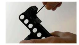
The thickness of your reflex optic determines which set of optic mounting screws to use. You want to use the longest screw that does not protrude below the lower surface of the shotshell carrier assembly. Use the supplied hex key to tighten the reflex optic to the shotshell carrier assembly using no more than 10 in-lbs of torque. A drop of purple or blue thread lock on each screw is highly recommended.
