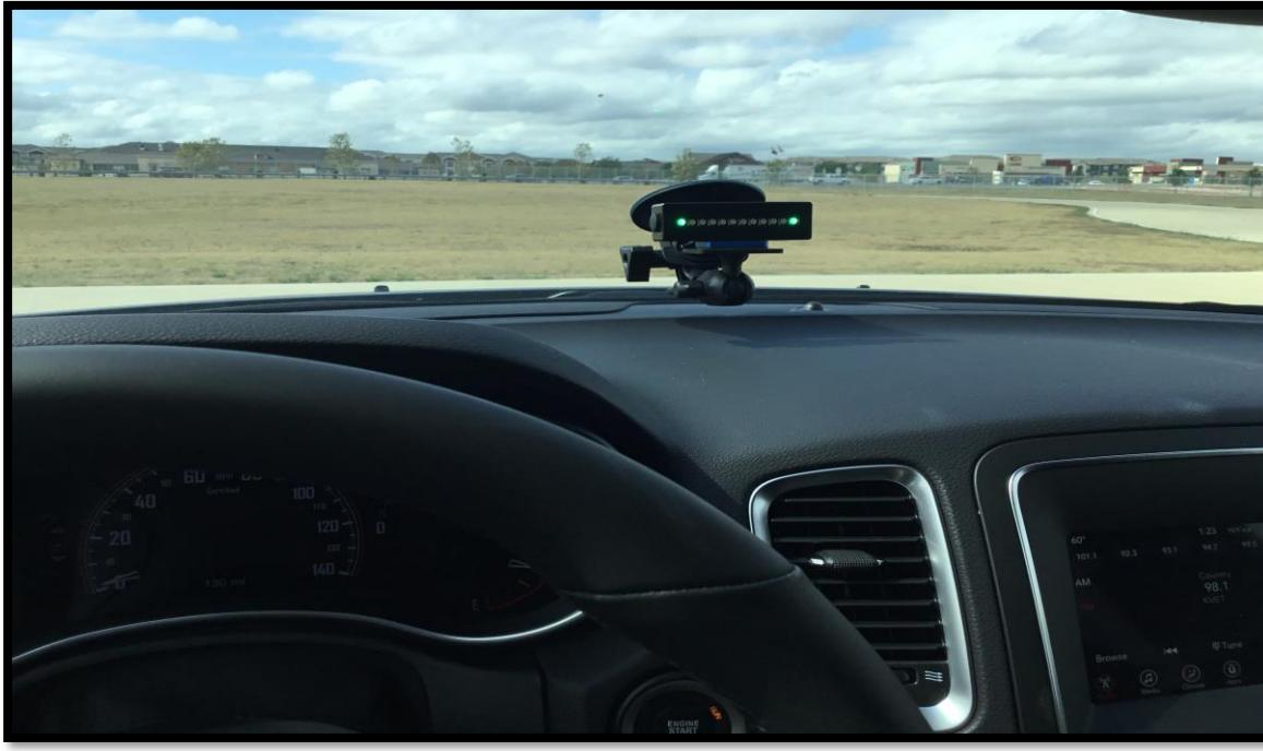
Additionally, the vehicles are equipped with a removable Apex Pro accelerometer. This electronic device provides immediate feedback to students through a series of red or green lights as well as the ability to monitor the device remotely using a mobile device such as an iPad. The Apex Pro will allow instructors to provide timely coaching to student drivers as well as self coaching through the use of its lighted display.
