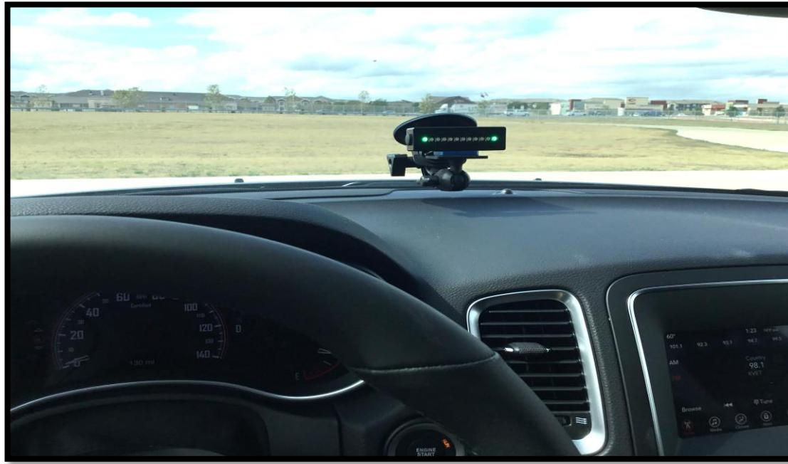
Additionally, the vehicles are equipped with a removable Apex Pro accelerometer. This electronic device provides immediate feedback to students through a series of red or green lights as well as the ability to monitor the device remotely using a mobile device such as an iPad. The Apex Pro will allow instructors to provide timely coaching to student drivers as well as self coaching through the use of its lighted display.
