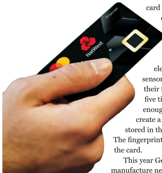
When the user inserts the card into the sleeve enough energy is created from ISO contacts connected to the card's chip to charge its secure element and fingerprint sensor. Cardholders move their finger on the sensor five times to capture enough information to create a template, which is stored in the secure element. The fingerprint data never leaves the card.
