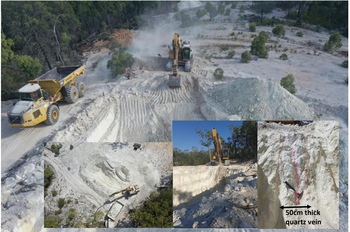
Mining at Surprise Pit where gold ore is being stockpile for treatment (red paint indicates veins)
