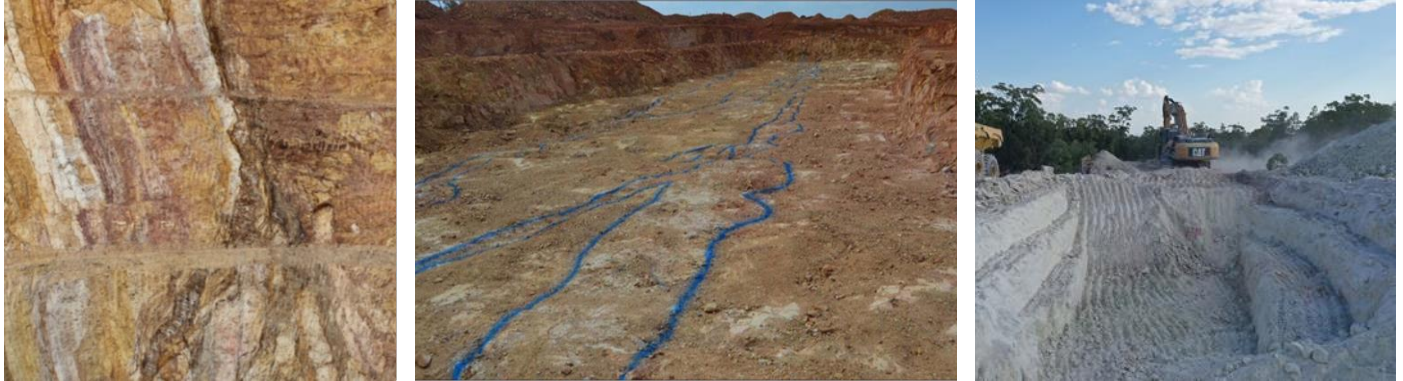
Targeted quartz lodes that hold the gold are quite visible and easy to follow via open cut
