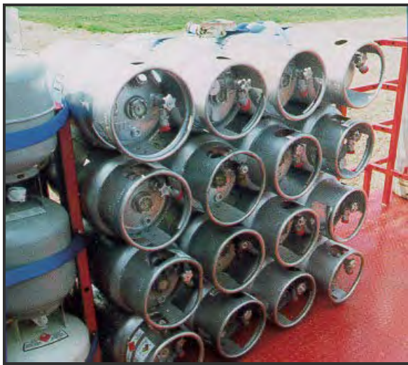
Figure 5.1.6c – Horizontally Secured Cylinders (Relief Valve at Top)
