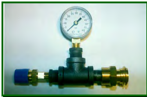
Figure 5.1.8f - Purging Adapter (POL to Male ACME)
