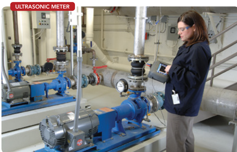
Figure 3. Clamp-on version can prove valuable for troubleshooting a wide range of flow issues.
